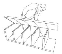
5) Position the second side wall so that each tongue fits into the grooves. Make sure the side wall and shelves are flush.
