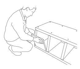
7) Press the former board into the upper compartment of the shelf unit. This serves to keep the shelf unit at right angles and is removed once the adhesive has hardened.
