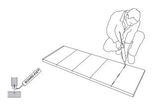
1) Apply adhesive to both joining parts (side wall and shelf).
