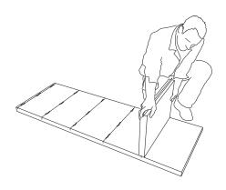
2) Insert the shelf into the groove on the side wall. Make sure the shelf and side wall are flush.
